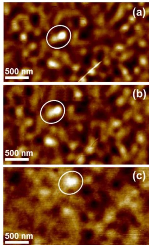
**Fig. 5.** AFM images of the topography of a-Se film placed on the Au NPs before irradiation (a). The ChG film thickness is 100 nm. The same area after irradiation with 650-nm laser beam ( $100 \text{ mW/cm}^2$ ) for 20 (b) and 70 min (c). Appropriate places in the circles were taken, and they illustrate initial surface topography and flattening of the film surface due to plasmon intensity distribution inside the glass matrix.
