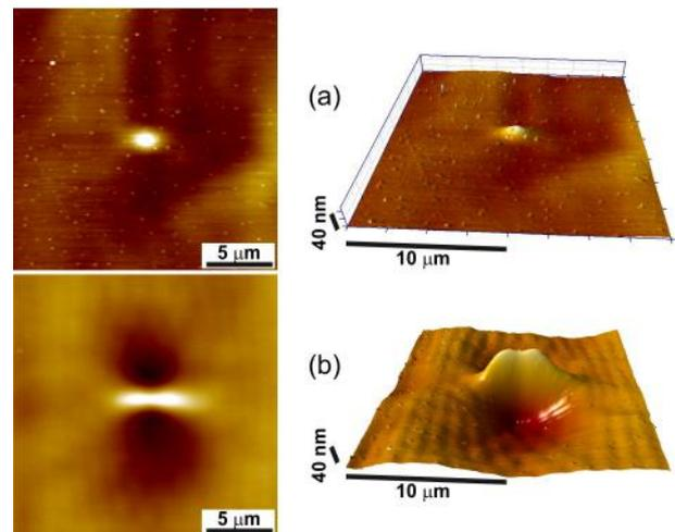
**Fig. 6.** AFM images of an isotropic expansion (a) and an anisotropic surface relief (b) in  $\text{As}_{20}\text{Se}_{80}$  film with thicknesses of 1  $\mu\text{m}$  after exposures of 10 and 2400 s, respectively, by linearly polarized light (2.0 eV). The polarization of the laser is oriented vertically. 2D and corresponding 3D images are presented.
