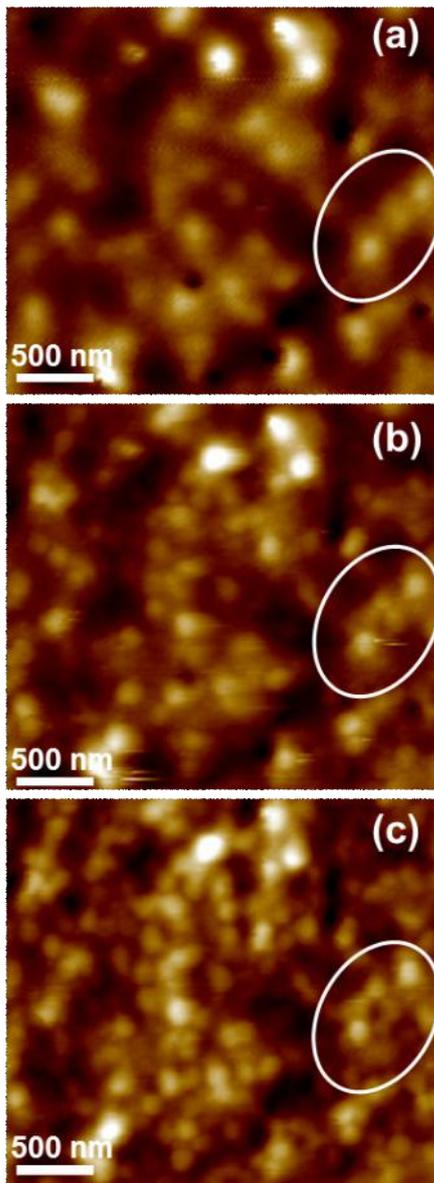
**Fig. 4.** AFM images of the topography of  $\text{As}_{20}\text{Se}_{80}$  film placed on the Au NPs before irradiation (a). The ChG film thickness is 100 nm. The same area after irradiation with 650 nm laser beam ( $100 \text{ mW/cm}^2$ ) for 5 (b) and 7 min (c). Appropriate places in the circles were taken, and these illustrate initial surface topography and surface relief increasing due to plasmon intensity distribution inside the glass matrix.
