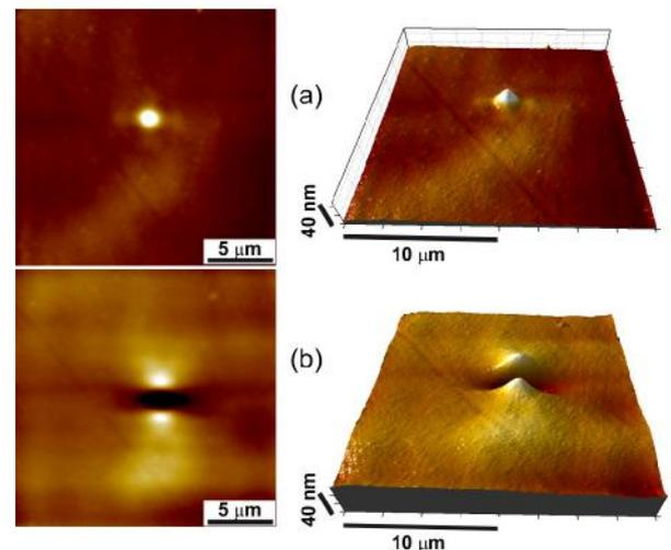
**Fig. 7.** AFM images of (a) an isotropic expansion and (b) an anisotropic surface relief in a-Se film with thicknesses of 1  $\mu\text{m}$  after exposures of 10 and 500 s, respectively, by linearly polarized light (2.0 eV). The polarization of the laser is oriented vertically. 2D and corresponding 3D images are presented.
