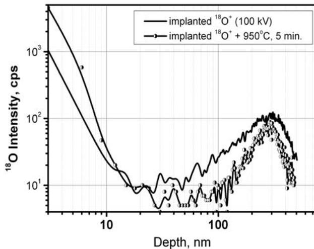
Fig.3. SIMS oxygen depth profiles after <sup>18</sup>O implantation in the arsenic-implanted structure before and after annealing at the temperature of 950°C for 5 min.
