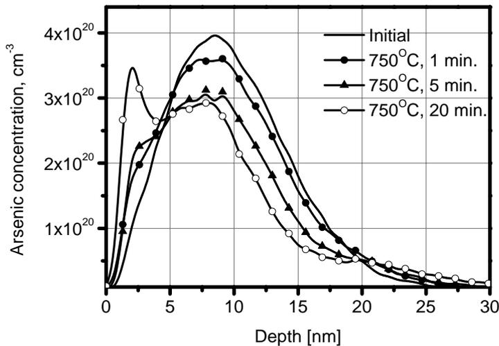
Fig.5. SIMS arsenic depth profiles before and after furnace annealing at 750°C for different times.
