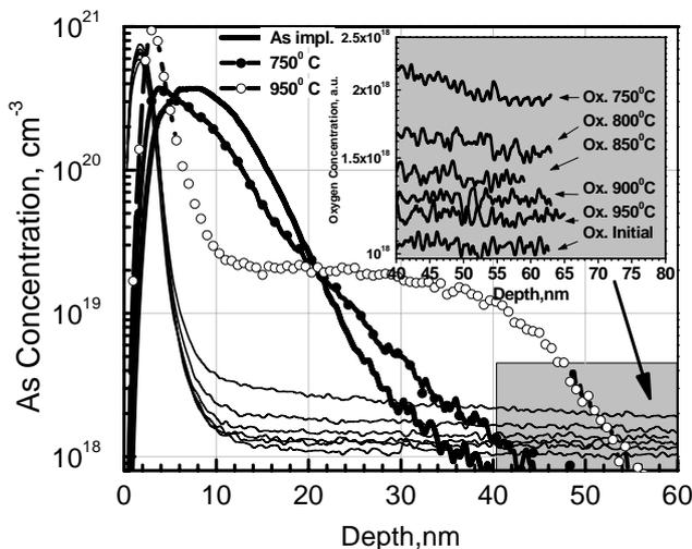
Fig. 1. SIMS depth profiles of arsenic and oxygen distributions at different annealing temperatures. Inset shows the change of oxygen concentration at the tail of arsenic depth profile after annealing.
