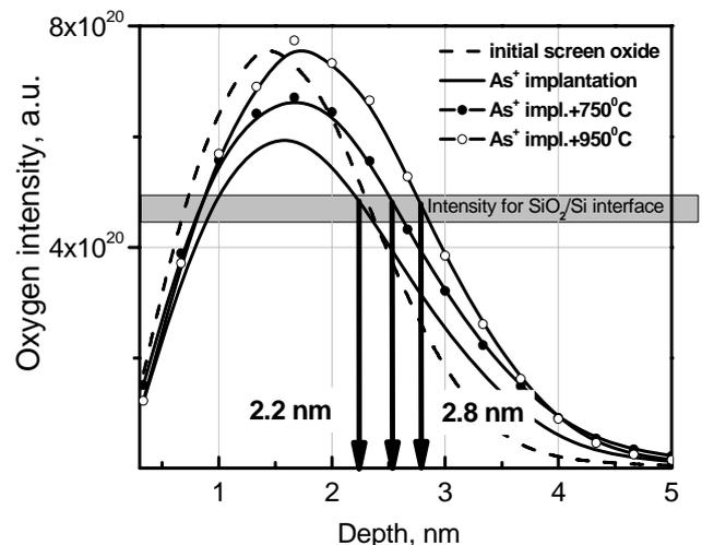
Fig. 2. SIMS depth profile of oxygen close to the SiO<sub>2</sub>/Si interface before and after annealing at different temperatures (5 min.)
