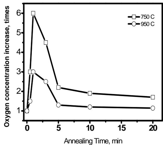
Fig.4. Time dependence of the relative oxygen concentration in the USJ region (10 – 50 nm) after furnace annealing.
